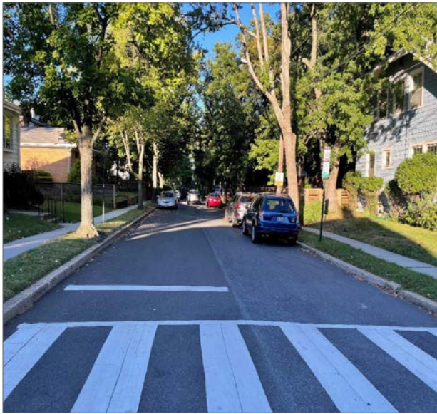
Figure 53. A yield street accommodates sidewalks on Walnut Street in northwest D.C. (PHOTO BY TOOLE DESIGN GROUP)
