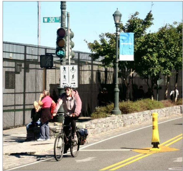
Figure 54. Bicycle and pedestrian signal heads queue riders and pedestrians at a signalized intersection in New York City. (PHOTO BY M-NCPPC)
