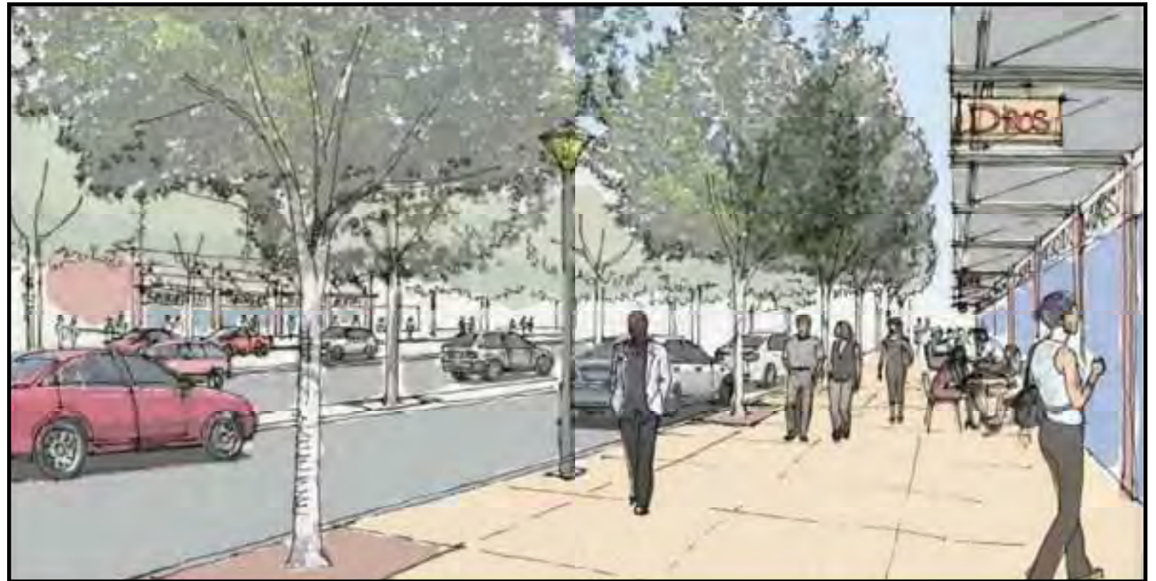
Sketch view of Silver Hill Road near its intersection with Navy Day Drive shows a protected slow lane, wide sidewalk, and urban-style storefronts.
