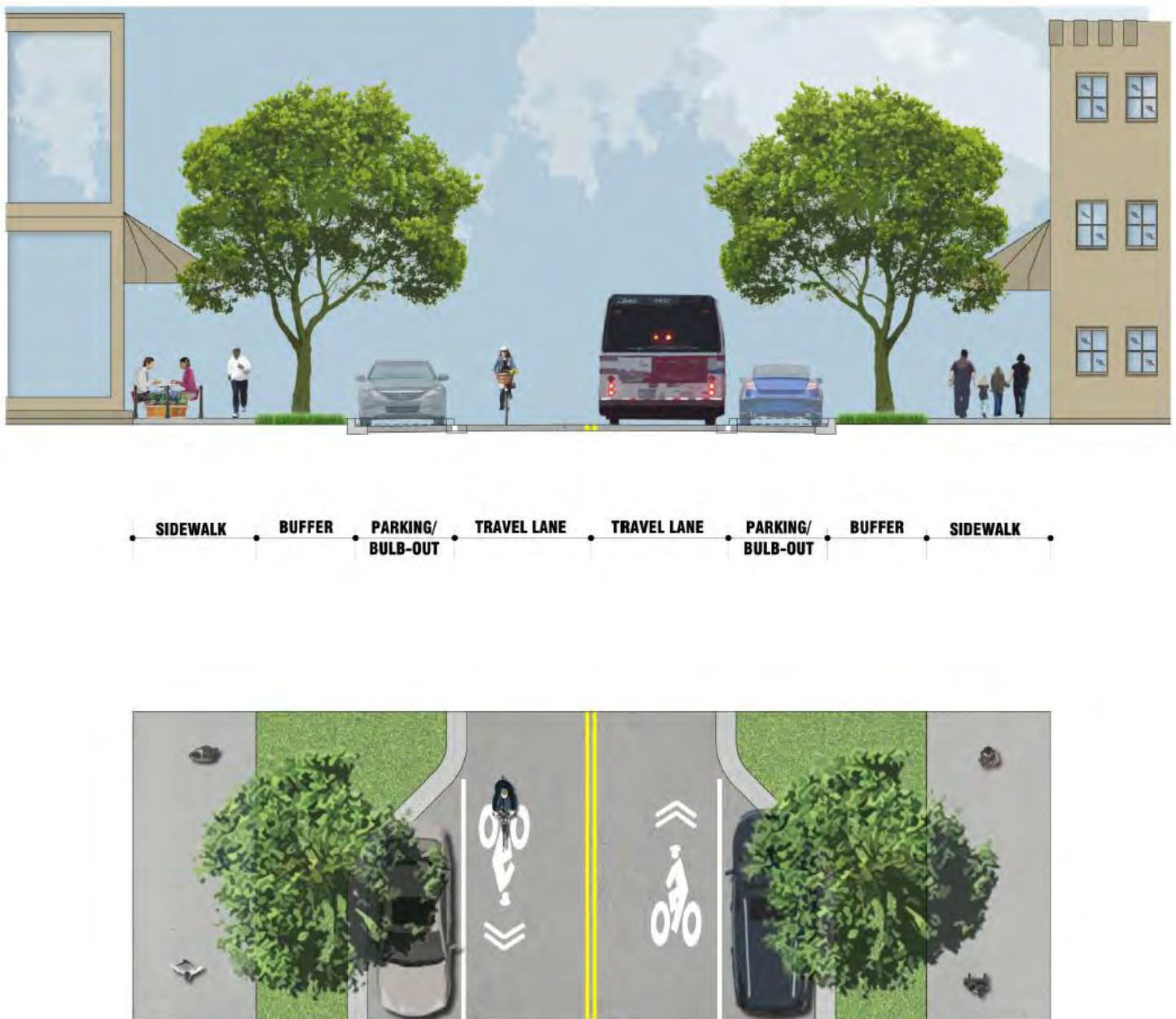
FIGURE 23. TYPICAL NEIGHBORHOOD COMMERCIAL CROSS SECTION
