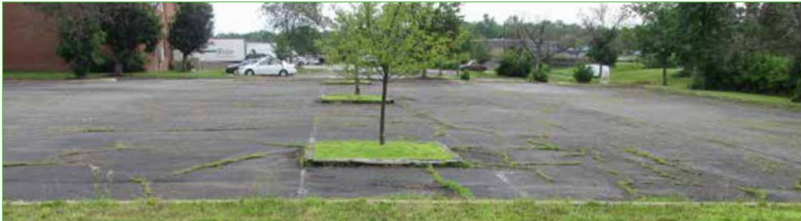
Large impervious surfaces contribute to the urban heat island effect and exacerbate stormwater management concerns in flood-prone areas.
