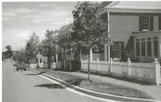
Residential streets in the town commons are proposed to include shade trees, sidewalks set back from the curb and on-street parking (Type II streets).
