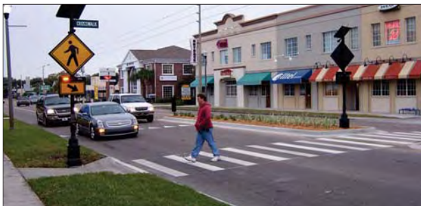
Rectangular Rapid Flash Beacon $12,000 - $15,000 for both directions Signs with a pedestrian-activated "strobe-light" flashing pattern that attracts attention and notifies motorists that pedestrians are crossing
