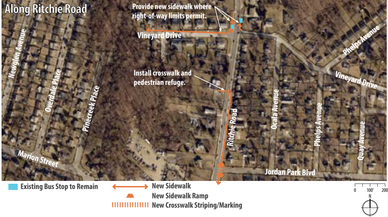
Figure 19. Locations Along Ritchie Road at Jordan Park Boulevard Design Concept Plan View
