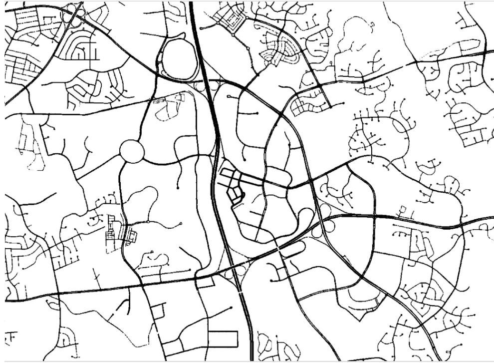
Street Network on Largo, MD. Largo is an island of dead-ends and loops surrounded by major arterial roads and culdesacs.
