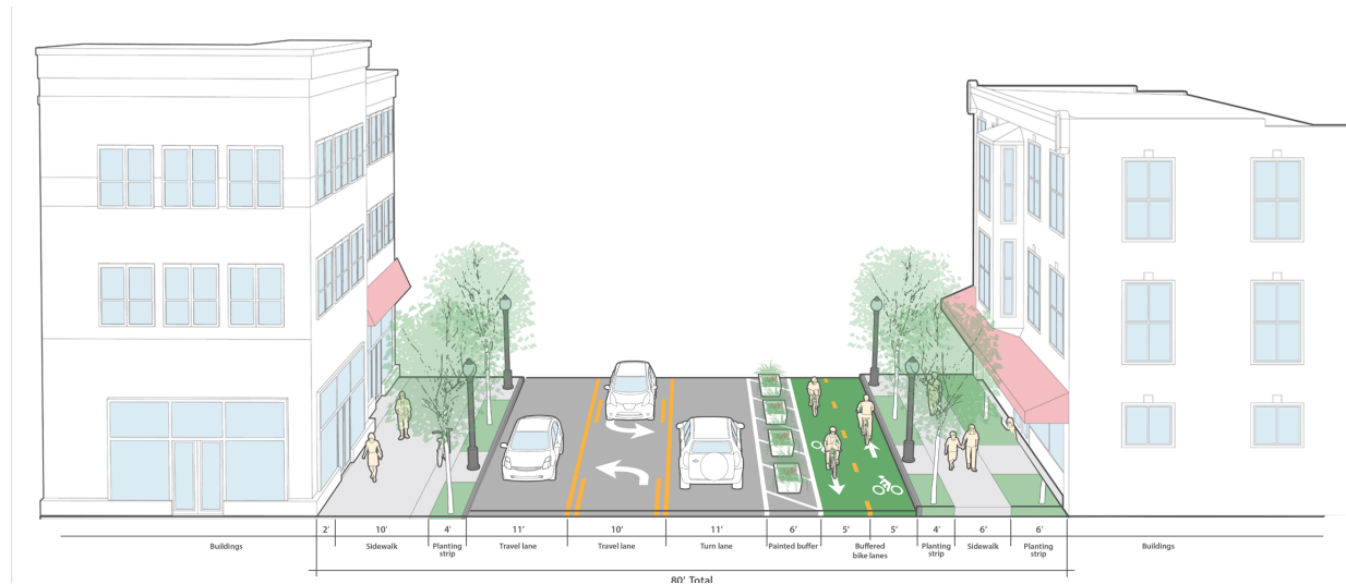
Figure 21. Livingston Road with Center Turn Lane and Painted Bike Lanes
